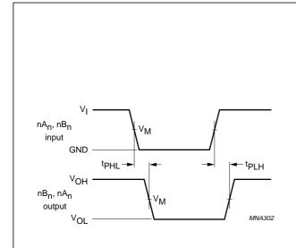
Fig.6 The inputs  $nA_n$ ,  $nB_n$  to outputs  $nB_n$ ,  $nA_n$  propagation delay times.
